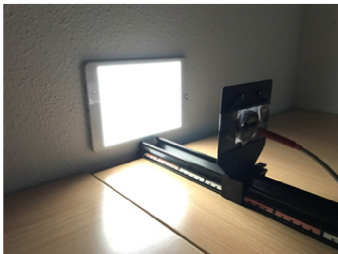
Figure 3: Spectrophotometer Ocean Optics USB 2000 installed on the optical bench was used to measure the screen's light emission.
